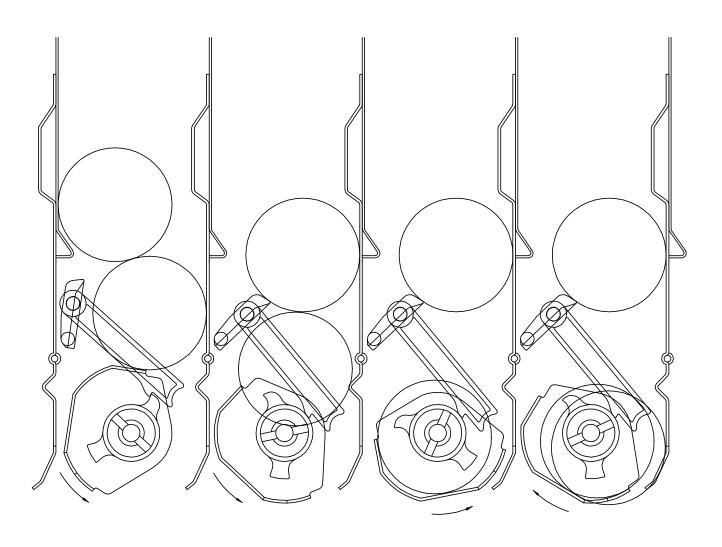
BUCKET ROTATES COUNTERCLOCKWISE CAM PUSHES LINK LINK OPENS GATE BUCKET CONTINUES COUNTERCLOCKWISE GATE CLOSES AS PRODUCT LOWERS INTO BUCKET BUCKET REACHES
